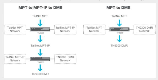
The TN9500 is able to connect multiple Tait networks allowing you to regionalize a single system into many sub-networks for more efficiency. For example, your maintenance is managed locally and the network is adapted to the geography of your operations.
