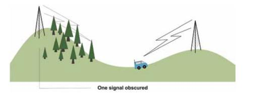
Simulcast transmissions take place from base station transmitters, so they affect the down link (talk out) performance of a communications system.
