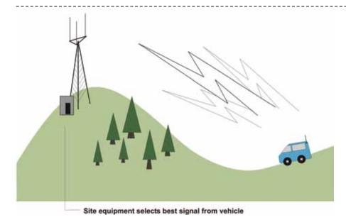
Micro Diversity combats the effects of the signal fading as a terminal moves through an urban area but it does not increase the coverage reliability in the same mathematical sense as Simulcast and Macro Diversity. Instead, it reduces the
