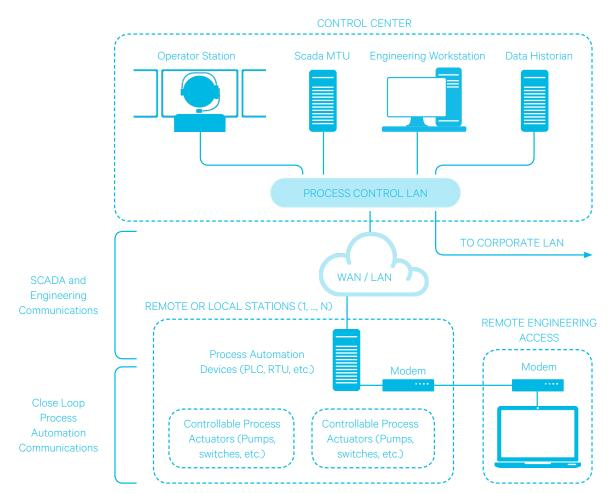
Data (meter readings, equipment status reports) are sent from a remote or local site to a control center where - by human or automatic intervention - supervisory commands can be sent back to the remote site. Controllers trigger actuators to change the operation of physical equipment at that site. Equipment can be remotely monitored and controlled, and its operation can be modified, turned on, or off.
