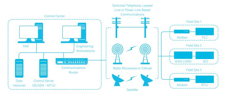
A specific example of this generic design is a Voice+SCADA system using Digital Mobile Radio (DMR) communications to connect a dispatch center, field maintenance crews, and an operator using the Human-Machine Interface (HMI) of the SCADA system.
